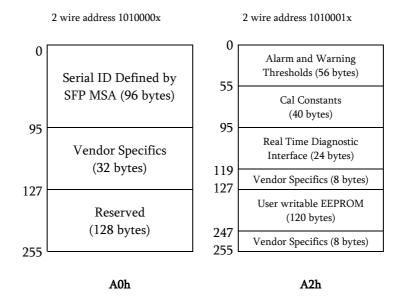
Figure 3. EEPROM of a an SFP
