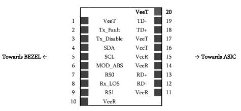
Figure 2. Transceiver Electrical Pad Layout
