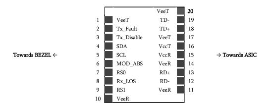
Figure 2. Transceiver Electrical Pad Layout
